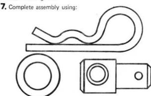
remaining Retainer Spring, Washer and Adjusting Pin found in bag of parts.
